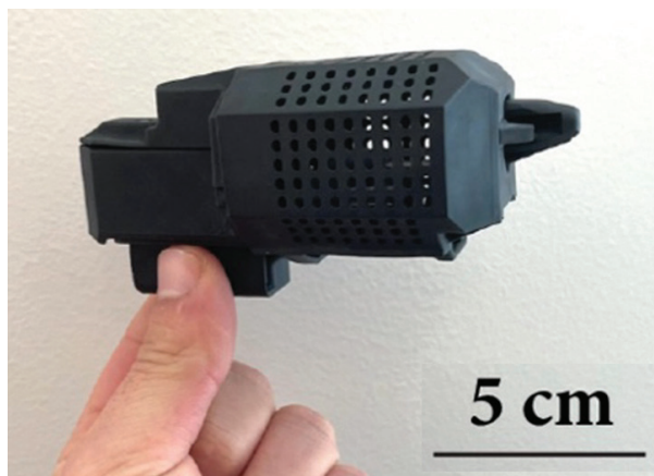
Figure 1: The microscope in a compact 3D printed housing.
